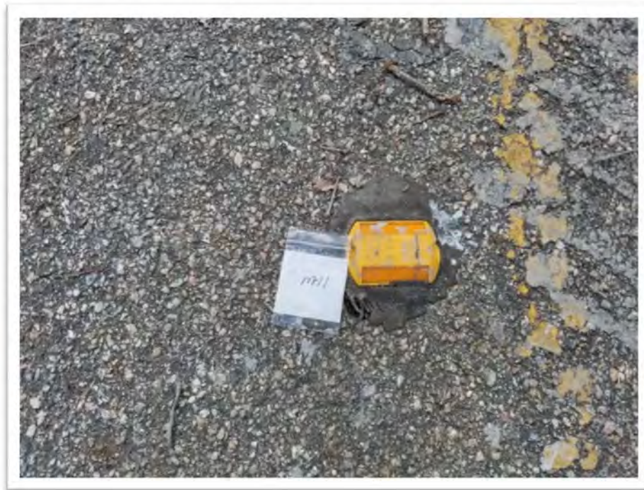
Photograph #22 Sample M-11 – Black Mastic Sampling Point at a Reflector on the Roadway of Bridge 3 (None Detected)
